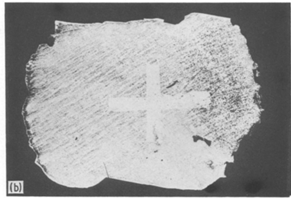
Figure 3 Dust patterns of boron-implanted region in colourless natural diamonds. (a) Two parallel bands on sawn surface. (b) Cross on polished surface.
